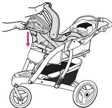
Position mounting notches over arm bar. Push down on car seat until the attachment latch snaps into arm bar.
